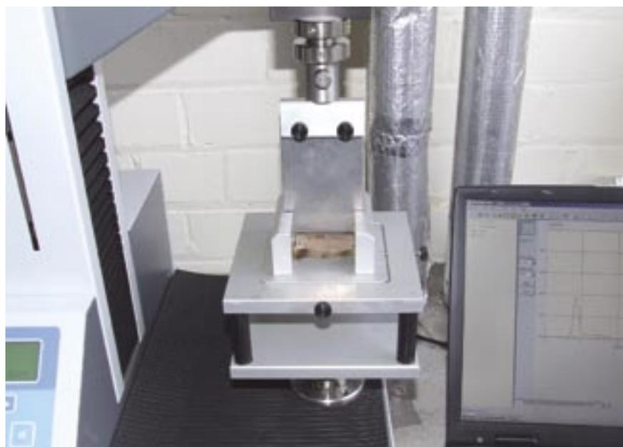
Figure 2: SAC custom-designed jig for rapid Slice Shear Force measurement
