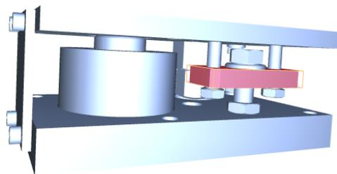
There is also lift-off protection built in, another feature that should always be considered with portable tanks or tanks mounted outside.
