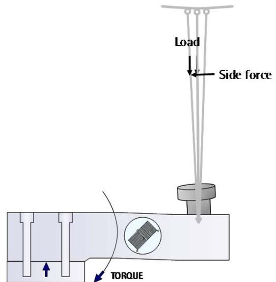
With the Rocker Pin, side force causes tilt and a restoring force compensates expansion/shear forces with less impact on accuracy. The canister load cell with a spherical element on both top and bottom gives the highest accuracy because it will not transfer side forces or moments.
