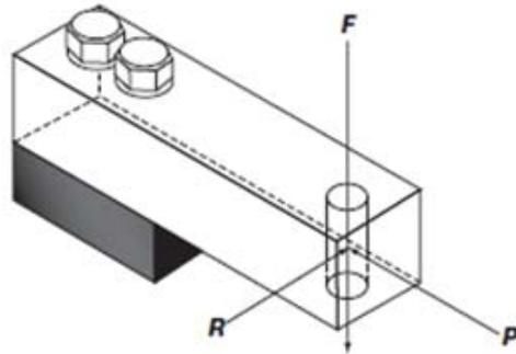
Hopefully the load will be from "F" direction. Suppose there is a thermal expansion between the Frame and the tank? A force "P" or "R" will be exerted on the cell causing the undesired output of the strain gage.
