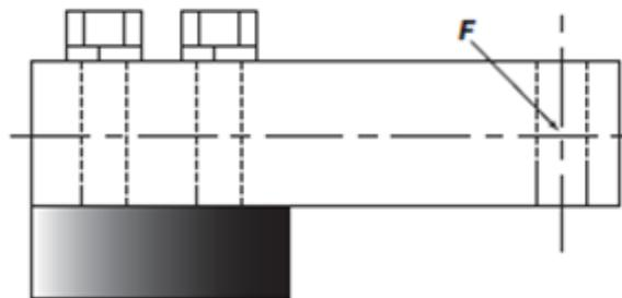
If the load is applied at an angle because of imperfect installation or design, the force will be reduced by the cosine error.
