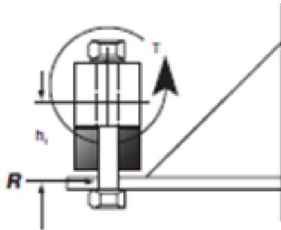
Sometimes when a side load is introduced the effect will be a twisting motion, again causing unwanted output from the strain gage.
