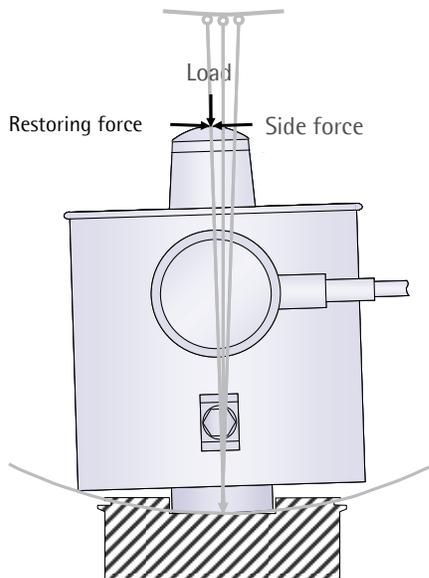
Shear Beam Principle:
