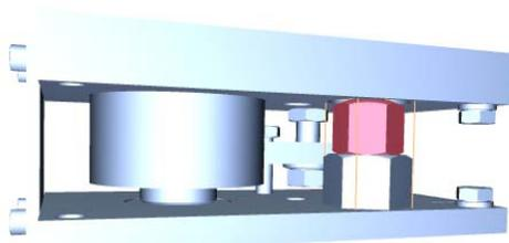
This load cell/mounting kit combination has an integral Jack-Up Mechanism. This allows load cells to be easily removed for maintenance or cleaning and to lift the load off of the cells for long range transport of the system.
