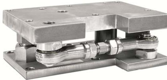
Here is a more compact design that incorporates the Lift-off protection feature that prevents a tank from tipping over and Jack-Up mechanism for taking the load off the load cell during transport or for maintenance operations. A constrainer is used to protect the load cell from unwanted horizontal forces.
