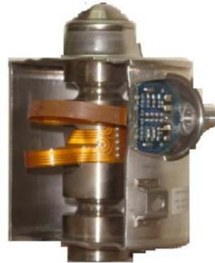
With this type of load cell the load introduction is centered for installations with as much as 2 degrees tilt. These load cells must be mounted in a "mounting kit" that will use constrainers to keep them in place in one direction, but allow the load cell to move in cases of thermal expansion.
