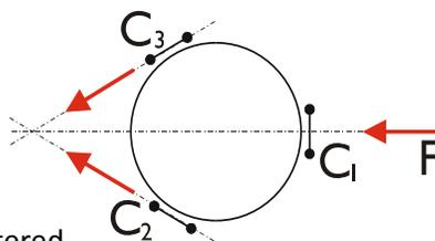
If only forces from one direction are expected, two constrainers in parallel will work very well, however, forces from other directions can cause problems.
