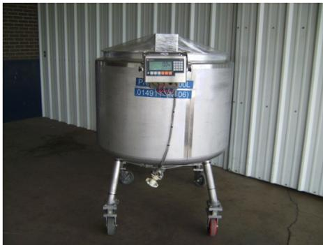
The nature of the caster swivel means that the load introduction is off-center with the loadcell measurement axis. Since the caster can come to rest at any angle, the loadcell needs to be designed to deal with substantial variable off-center loads.
